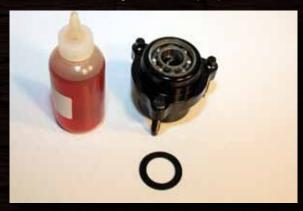
tion is just as simple. Using a solid block of metal or wood, drive the bearing solidly into position. Some of the new design front hubs allow you to remove a single snap ring and you can replace the bearings without any additional tools. This also eliminates any crush on the bearing, further decreasing drag.
