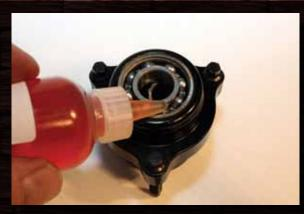
bearing oil circulated through each bearing is sufficient, and you can snap the seal back into place. I personally recommend removing the hubs before washing the kart and keeping them away from water. The water tends to accumulate in the area between the two bearings and greatly shortens bearing life.
