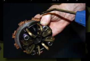
blow the center section enough to remove all dust and particles from within the clutch. On occasion, brake cleaner can be used to assist with this, however I don't believe in using it weekly, and carb cleaner should not be used. Carb cleaner is more aggressive than brake cleaner, and can attack the cement than holds the friction material to the plates and that can lead to more problems.
