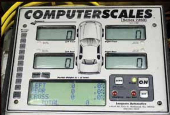
Check and adjust the chassis to achieve the weight percentages based upon recommendations and the expected track conditions. Have the kart "track ready", all fluids and items just as it will be on the track. I prefer to get the left side, and nose weight close, then adjust the cross
