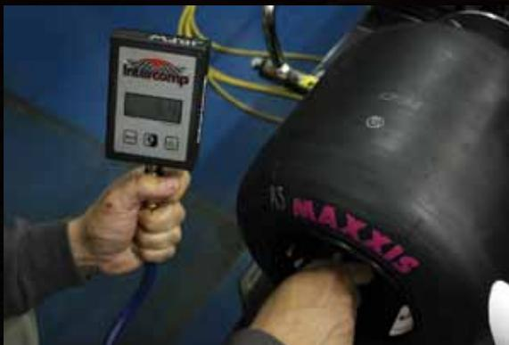
tion pressure and adjust. Use a pressure you expect to use at the track; nothing to an extreme high or low, just a good neutral setting. Before tightening up, take a quick minute to inspect the wheel studs. Make sure the threads are good, and verify they are tight into the hubs. Check the lug nuts for good edges, a rounded off lug nut can be a major issue.
